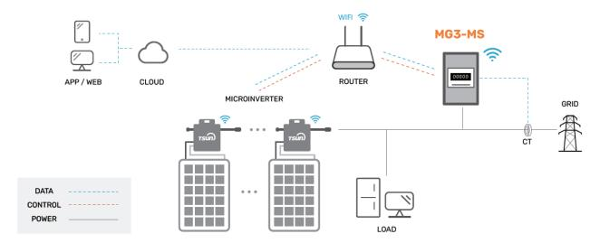
The microinverter converts the DC electricity generated by solar panels into AC electricity which is in accordance with the requirements of the public grid and sends the AC into the grid, reducing the load pressure of the grid.
