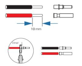
**Tips:** Use AWG 12 (or 4 mm<sup>2</sup>) cable for DC cable.
