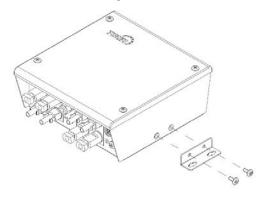
Step 2: Fix the rapid shutdown control unit
