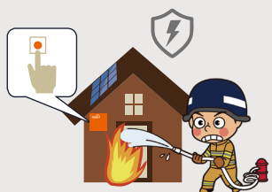
Rapid shutdown control unit cut off solar power automatically or manually, no life risk put out fire using water, firefighter can work now.
