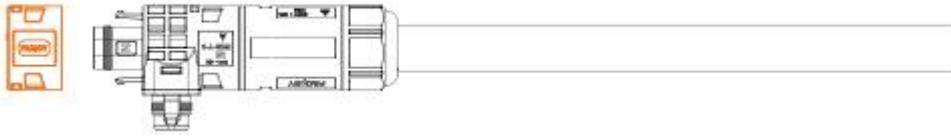
Fabricate the AC end cable. Insert the connector of the end cable into the T-connector, and connect the other side to the distribution box.
