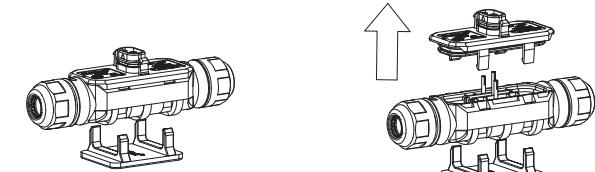
Insert AC trunk cable into T connector .Tighten T connector.
