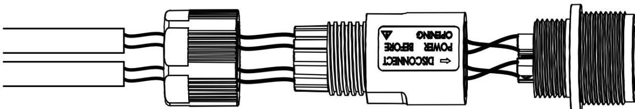
Plug the four core connector into the microinverter communication terminal and connect the four core connector to the RS485 connector.
