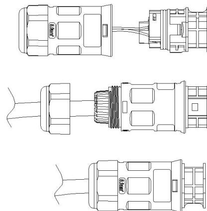
Plug the AC connector into the micro inverter and connect the AC cable to the AC distribution box.
