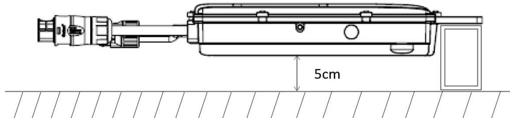
Choose the best installation position. Use two pairs of screws and nuts to fix the micro inverter on the frame. Make sure that the label of the micro inverter should be the upside.
