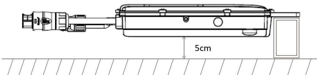
Choose the best installation position. Use two pairs of screws and nuts to fix the micro inverter on
