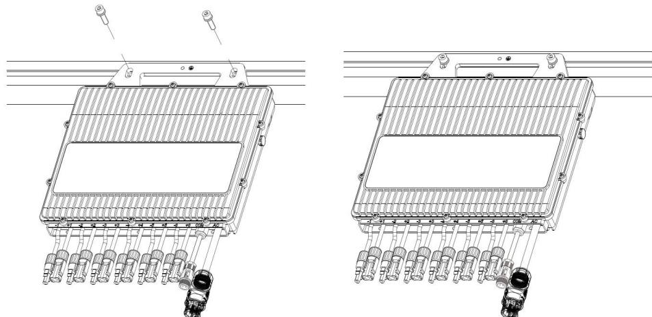
The micro inverter can also be mounted on the wall (vertically) using the optional support. In this case, first, fix the bracket to the wall with a pair of screws, and then fix the micro inverter to the bracket with one pair of nut screws.
