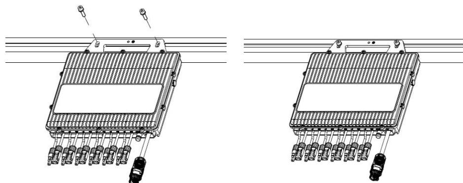
The micro inverter can also be mounted on the wall (vertically) using the optional support. In this case, first, fix the bracket to the wall with a pair of screws, and then fix the micro inverter to the bracket with one pair of nut screws.
