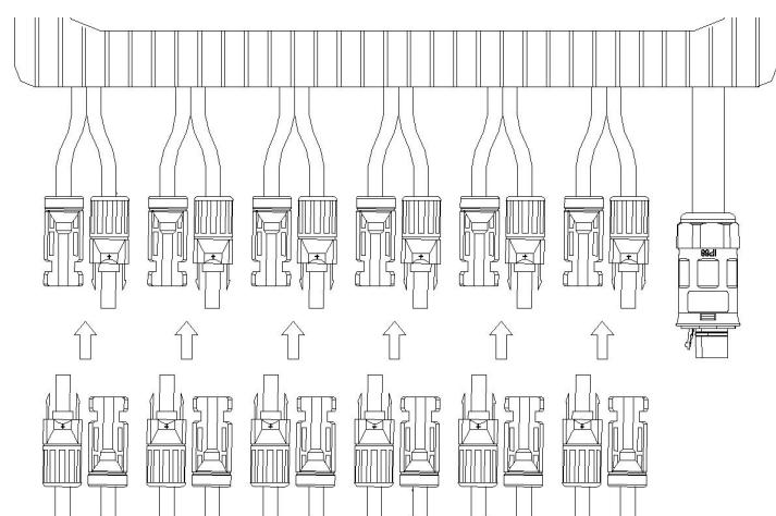
While using TSOL-MS3000 micro inverter, each DC input of micro inverter can connect two PV modules in series.
