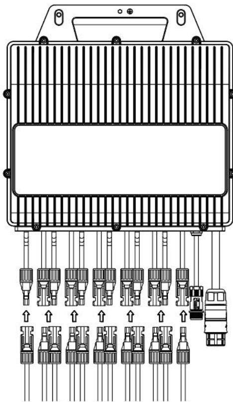
While using TSOL-MS3000 micro inverter, each DC input of micro inverter can connect two PV modules in series.
