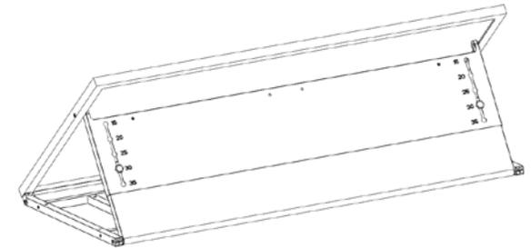
Use a hex wrench (#5) to open the angle locks. Slowly put down the solar panel and make the angle locks slip into the right angle. Then tighten the angle locks again.
