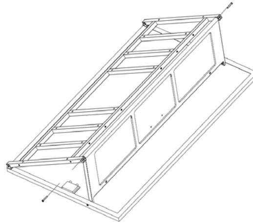
**Warning:** The bracket must be fixed on the base plate, which will promote the wind loading rating of Easy Solar Kit.
