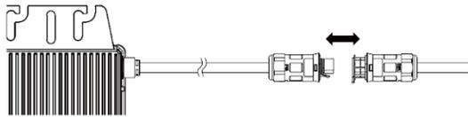
Connect the two sides of extension cable to the microinverter and the end cable.
